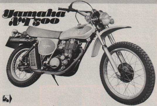
test the XT's units remained at their softest, smoothing out the roughest roads with no trace of bottoming or jarring. Up front, the tele. forks were rather spongy for fast road work, although I understand there are two rates of internal springing — first soft, then hard — to cope with on and off-road going.
