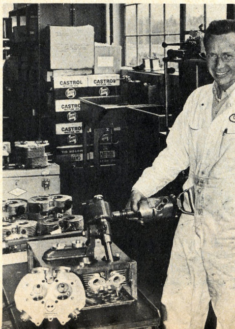
Doing a little relieving — Cliff Guild uses a high speed Die Grinder to open up the intake ports to the prescribed 1\frac{1}{8} " diameter. The Triumph Corporation offers to rework Tiger 100 cylinder heads as part of its many services to dealers.
