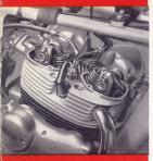
Simple and positive valve adjustment is provided by eccentric rocker spindles in the polished alloy head
