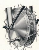
Front Hub: full width 8" dia. in lightweight polished alloy, extremely efficient and well ribbed for quick heat dispersal.
