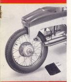
The rear wheel is easily withdrawn when the quickly detachable rear number plate has been removed.
