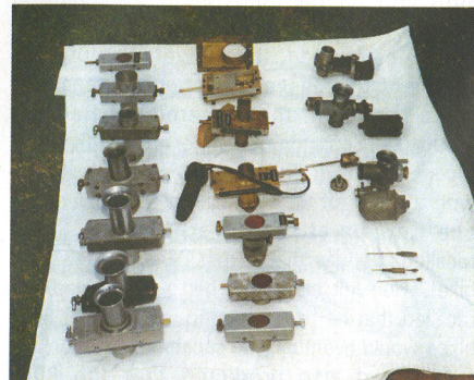
Bottom right is water/fuel injector; bottom left is a 1990s reproduction of a 1950s C-type carburettor.
